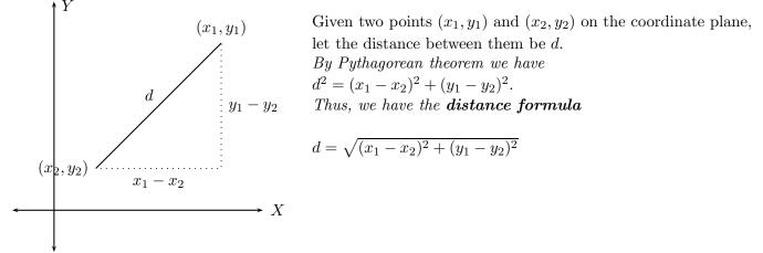
For example, to find the distance between points (2,3) and (-1,4), we first set  $(x_1, y_1) = (2,3)$ and  $(x_2, y_2) = (-1, 4)$ . Then, the distance d is given by
