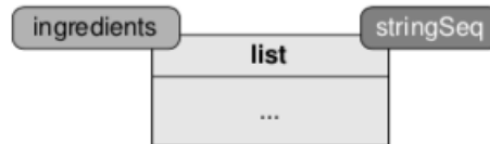
FIGURE 5.2: The parameter is identified as ingredients from the context of the caller, yet as stringSeq within the context of the function body.
