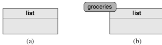
FIGURE 2.1: The steps in the execution of the groceries = list() statement: (a) creation of an empty list instance, and (b) the assignment of identifier groceries to the newly created object.
