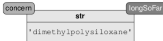
FIGURE 5.3: The mechanism for passing a return value is similar to that for a parameter. Upon return, the caller's identifier concern is associated with the object identified internally as longSoFar .
