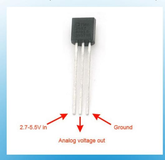
Temperature sensor TMP36 changes its voltage output depending on the temperature of the component.
